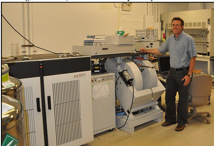
Dr. Randall with the Bruker EleXsys E-580 EPR spectrometer that operates in CW and pulsed mode at X- and Q- band frequencies. Dr. Randall used this instrument in his research at UC Davis during the summer of 2010.
