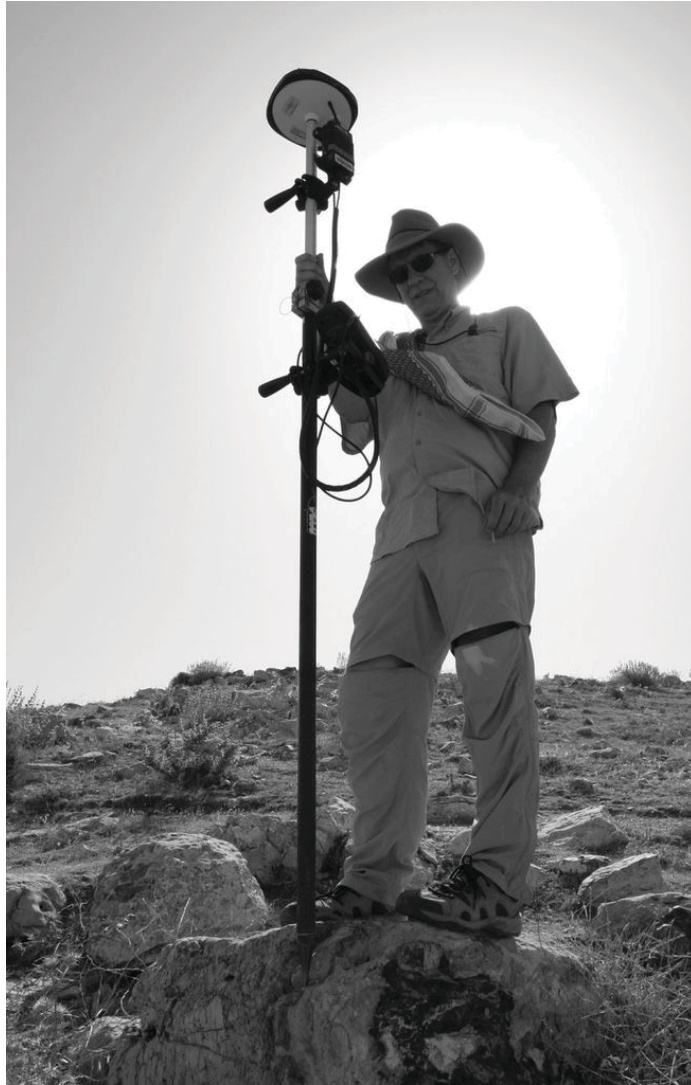
Figure 28. Robert Bates uses the Promark 3 GPS rover to survey walls on the western slope of the tell.
