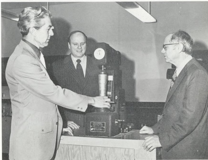
A surface hardness tester, used in machine and tool design to discover the hardness and strength of materials, is demonstrated by Dr. William W. Davidson (left), newly appointed dean of the College of Technology at Andrews University. With him are Dr. Richard Hammill (right), AU president, and Dr. Joseph G. Smoot, vice-president for academic administration. The College of Technology will begin operation in September, 1974, and will offer both two-year associate degrees and four-year baccalaureate degrees in industrial and engineering technology. Shorter programs leading to certificates in various areas of occupational education will also be available.
