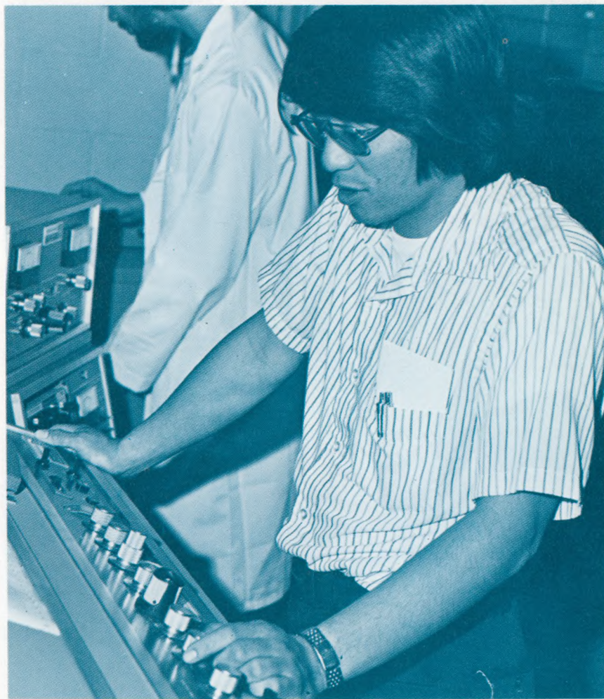
Norman Fojimoto (front) and John Ratzlaff, measure the absorption of ultrahigh-frequency radiation in a magnetic field using an NMR spectrophotometer.
