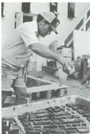
When the glass pieces were in place, a wooden frame was placed around the design. Shingle granules were sprinkled on the pattern to add texture, and finally epoxy was poured on to fill the spaces between the glass.
