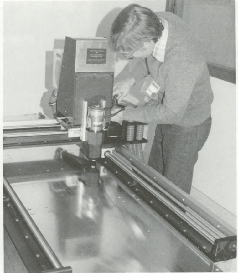
Building the computer numerical control machine drill at EDCO.
