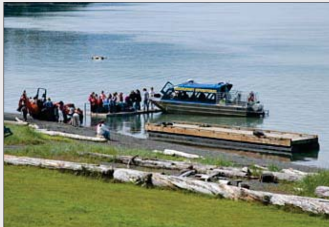
Campers arrive by boat ready to enjoy a week of summer fun. Due to the constantly changing tide, the camp uses a trailer as the dock. The stable water bottom allows a trailer/dock to be wheeled out to a safe depth for the boats and then pulled back to dry ground.
