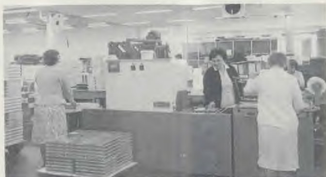
This picture shows the machine located in the bindery which seals the final products in an air-tight plastic wrap.
