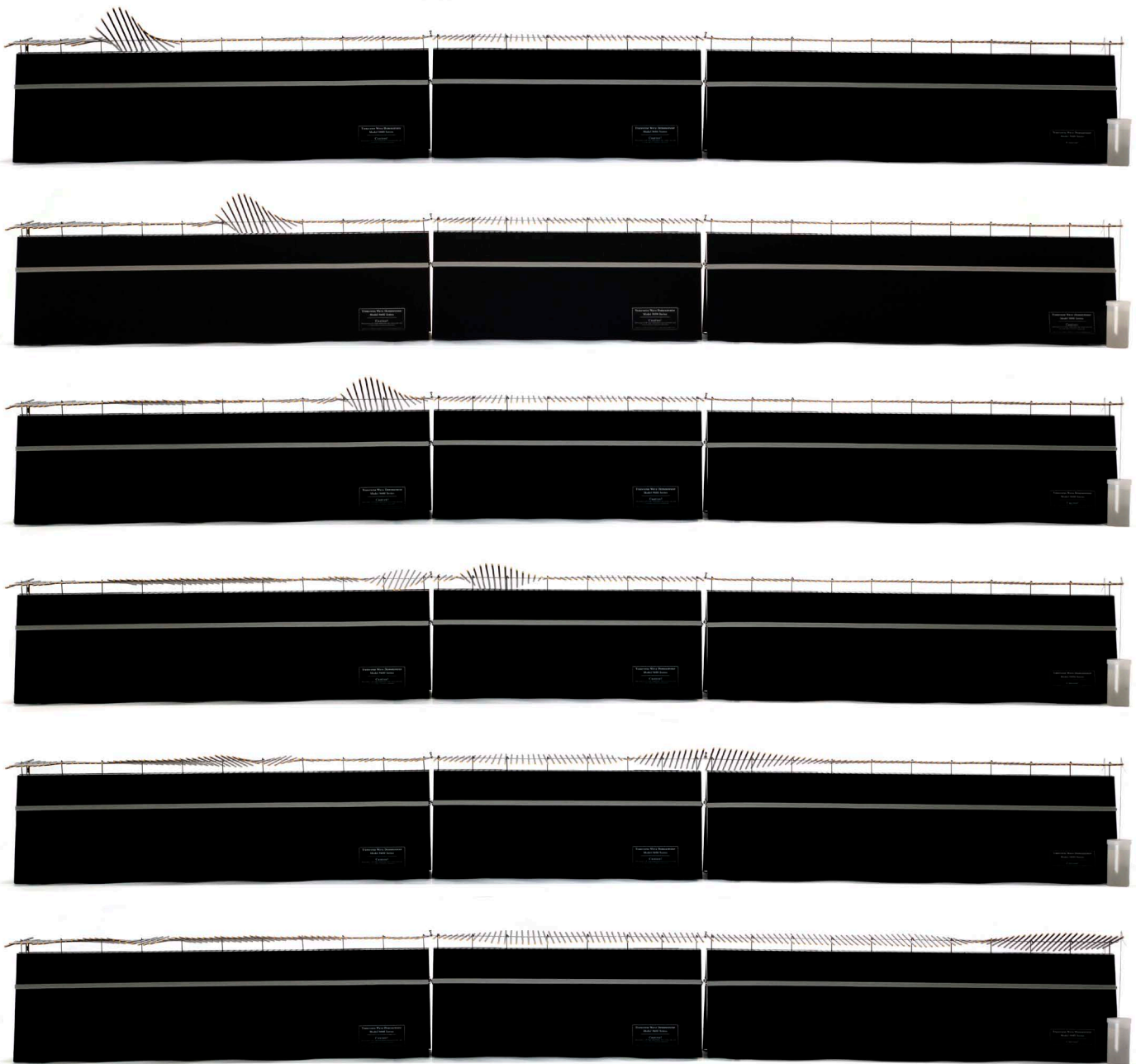
Figure 18. The same positive pulse as it travels to the right beginning on the wide demonstrator, traversing the tapered unit, and moving on to the narrow unit. The pictures were taken at 0.5s second intervals. Note how the pulse waveform speeds up and spreads out as it moves onto the narrow demonstrator as expected.
