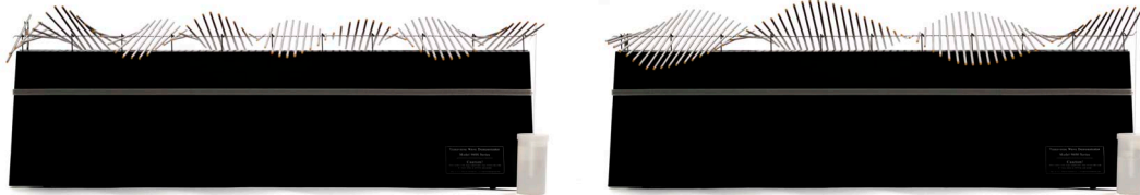
Figure 7. The wide wave demonstrator excited by a higher and a lower frequency periodic waveform (2 Hz and 1 Hz, respectively). For the 2-Hz excitation, the wavelength is about 20 bars, and for the 1-Hz excitation, the wavelength is about 40 bars.
