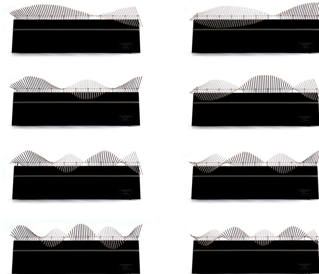
Figure 14. Standing waves with a node at the near end and an anti-node at the far end. Modes 2, 3, 4, and 5 are shown.
