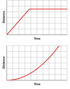
11. The data points from each tube follow <u>straight lines</u>. Straight lines have constant slope, and since the slope was the speed, the speed was constant.
