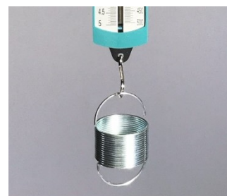
Fig. 6: Weigh the spring on the spring balance.
