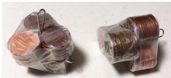
Fig. 16: Two hanging weights with 50 pennies in each.
