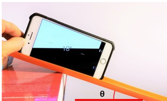
Fig. 6: Using a smartphone to measure the angle of inclination.
