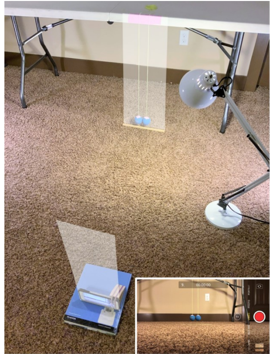
Fig. 6: Smartphone with wood block stand facing the pendulums and framed to place the racquetballs in the center of the image and the ruler in view below.
