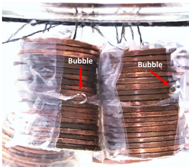
Fig. 5: Notice how bubbles trapped between the coins and the tape start to escape when submerged in water. Encourage all/most of the bubbles to dislodge and rise to the surface before weighing the pennies in water. If you do not, the air will increase the buoyancy of the pennies and introduce extra error into the experiment.
