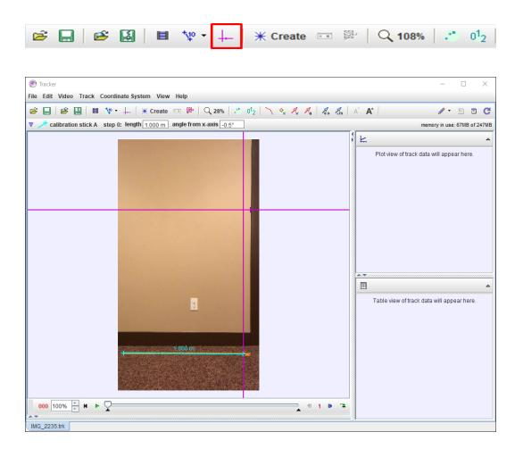
2. Move the axes to line up with the horizontal and vertical lines in your video. If the reference lines in your video are rotated a little bit, grab the positive x-axis and rotate the axes to match the video.
