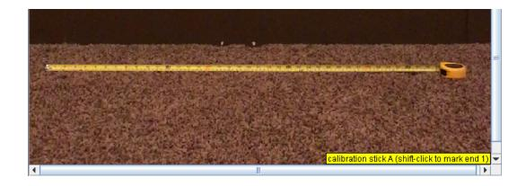
3. Type in the provided box to change the length of the Calibration Stick. Enter the length of the physical object. In this example, the measuring tape was set to 1 meter, so you would set the Calibration stick to 1 meter.
