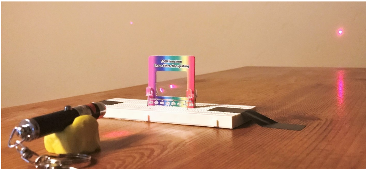
Fig. 6: Shine the laser through the diffraction grating at a wall. Tape down the grating to prevent it from moving.
