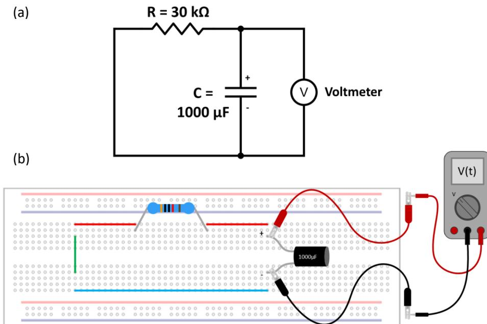
Fig. 7: RC Discharging Circuit - (a) Circuit Diagram and (b) Breadboard wiring diagram with multimeter (acting as a voltmeter) connected in parallel to the capacitor using alligator clip wires. In this diagram, a green jumper wire is bridging the gap where the battery was. Note that it does not need to be in the same holes that the battery wires were, but each end needs to be in the same row of 5 holes as the top and bottom jumper wires that it is connecting.
