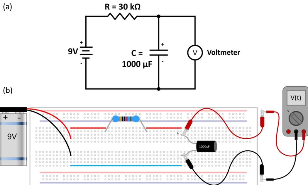
Fig. 5: RC Charging Circuit - (a) Circuit Diagram and (b) Breadboard wiring diagram with multimeter (acting as a voltmeter) connected in parallel to the capacitor using alligator clip wires. Make sure any wires/leads that should be connected are placed in the same row of 5 holes. Pay attention to the capacitor polarity (+/-). Remember that the longer lead is positive.
