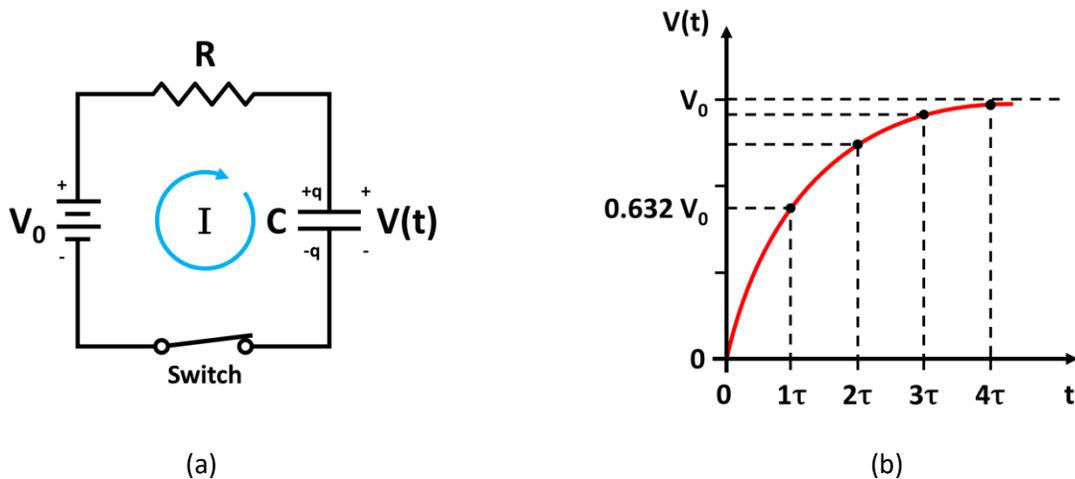
Fig. 1: (a) Circuit for charging a capacitor. (b) Plot of voltage vs. time for a charging capacitor.
