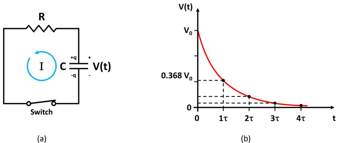
Fig. 2: (a) Circuit for discharging a capacitor. (b) Plot of voltage vs. time for a discharging capacitor.
