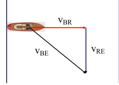
$\vec{v}_{BE} = \vec{v}_{BR} + \vec{v}_{RE}$ Add vectors by breaking into X and Y components
